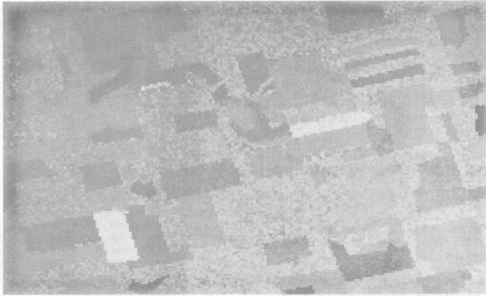
Figure 1. Simulated thematic mapper (TM) scene of spring wheat segment; blue, green, and red = channels TM-2, -3, and -4.
