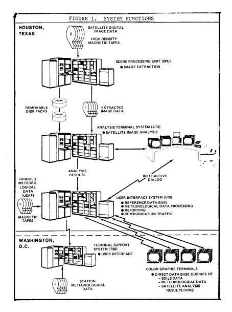
universal format for access by the analyst terminal system; METSAT images are recorded on removable disk packs. No digital imagery is stored in the CADRE database.
