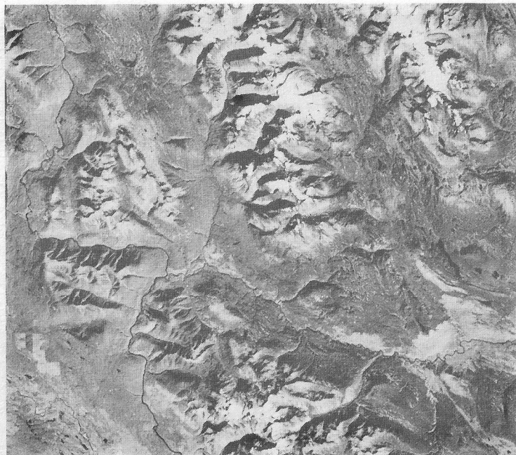
Figure 13. Simulated off-nadir (slant angle 27^{\circ} from right) MSS band 7 over Skeena Mountains, sub-scene from frame 57-21. Original scale 1:500 000.
