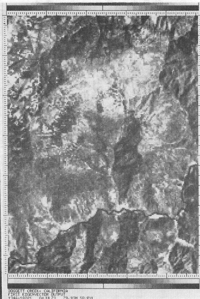
Figure 3. - EIGEN 1. The principal component (Eigenvector 1) of Landsat PCA highlights the reflectance differences between spectral channels due to wavelength, and therefore contains only marginal vegetation information.
