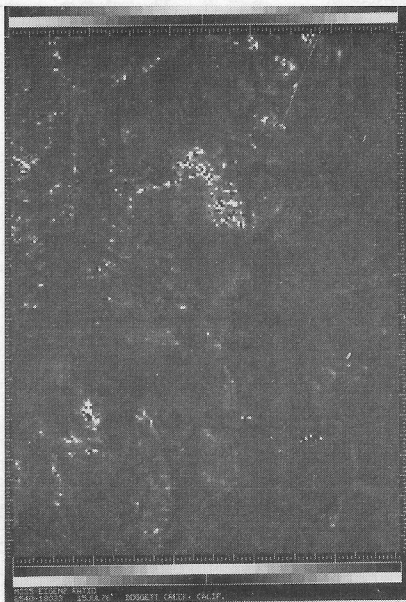
Figure 1. SATURATED PIXELS. MSS5/E2 unenhanced transform channel showing the saturated white and black pixels that occasionally occur when Landsat data is divided by the second principal component. Saturated pixels represent areas of unusual contrast between Landsat bands. Any saturated pixel falling into a training site used for divergence analysis would significantly alter statistical means rendering the technique unreliable.
