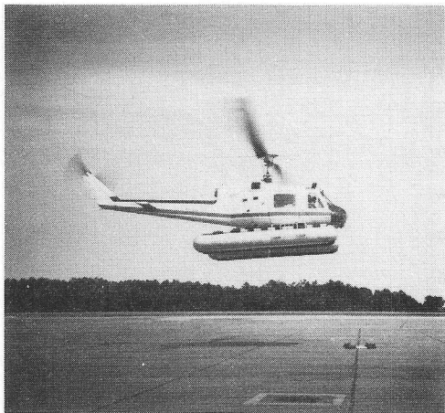
Figure 1. Photograph of the Bell UH-1B Iroquois (HUEY) helicopter used as a data acquisition platform. This photograph was taken as the pilot attempted to hover over a barium sulfate reference panel (weighted down with sand bags) at the beginning of our check-out mission.
