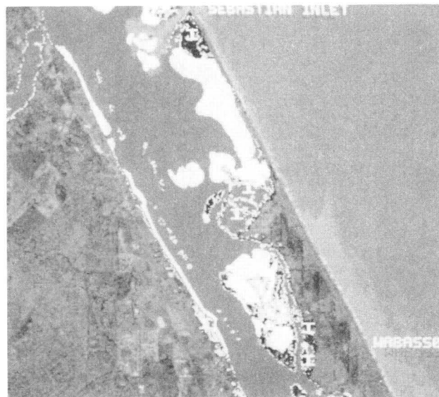
Figure II. A statistically processed TM image of a 12 km site in Indian River, Florida. Mangroves are depicted in black and seagrasses in white. Seagrasses were interpreted from 1984 aerial photography and imbedded into this 1982 image.
