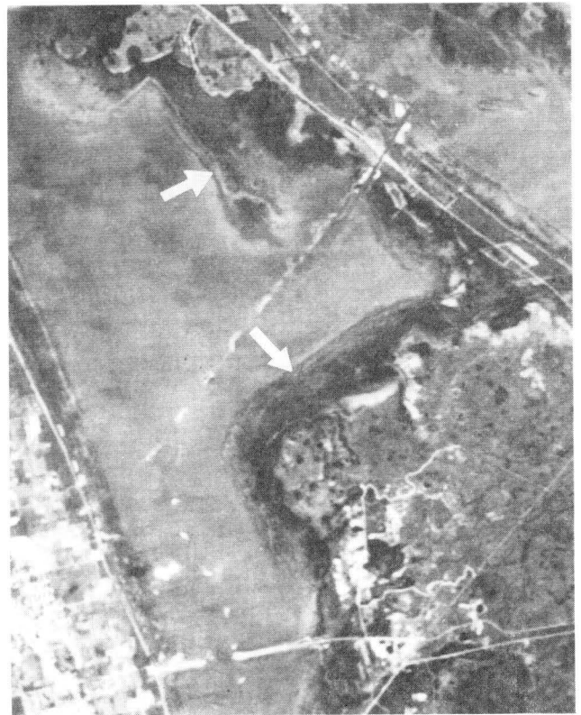
Figure 1. A 1984 TM image (channel 1, .45-.52 \mu\text{m} ) of a site near Cape Canaveral, Florida. Submerged vegetation (dark) is easily observed along the shoreline.
