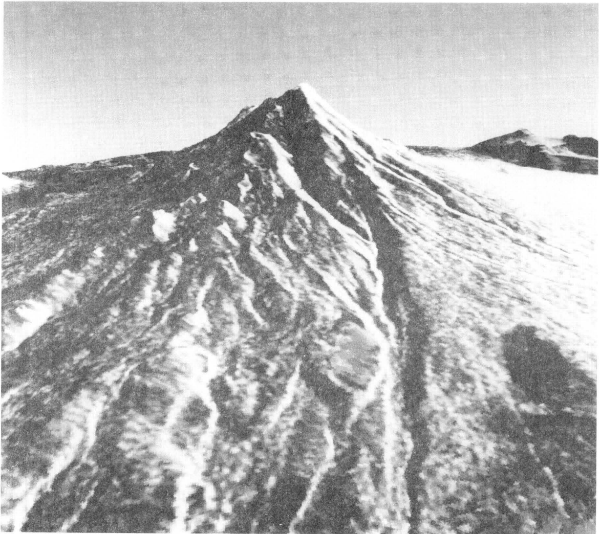
Figure 5b. A digital topographic data set can be used to generate a computerized perspective view such as this one of Mount Shasta. Any viewing geometry can be used, assisting in the visualization of morphological features, especially in remote areas.
