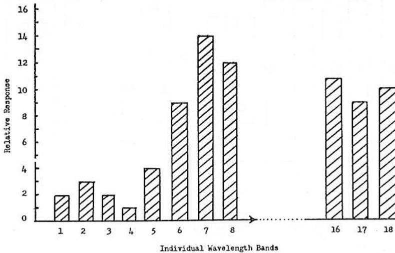
Figure 4. An illustration of a multispectral response signature which can be obtained through the use of eighteen wavelength bands of imagery. The current computer system allows a single wavelength band to have up to 16 levels of response. Data from a combination of 18 wavelength bands can therefore yield up to  $16^{18}$  unique multispectral response signatures.
