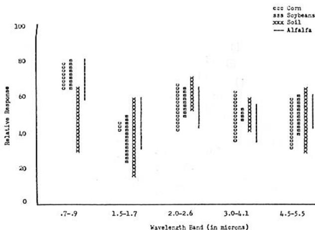
Figure 7. The distribution of the relative response within individual wavelength bands for corn, soybeans, alfalfa and bare soil. (Taken from flight data obtained at 1055 hours on 27 August 1964.)
