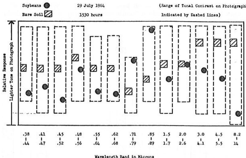
Figure 5. A multispectral response comparison between soybeans and bare soil, in relation to the total tonal contrast of individual wavelength bands of imagery.
