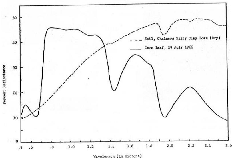
Figure 3. Spectral reflectance of a green corn leaf compared to Chalmers silty clay loam soil, as obtained on a Beckman DK-2 spectrophotometer.
