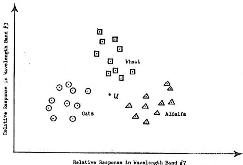
Figure 6. Hypothetical example of relative response of oats, wheat, and alfalfa in each of two wavelength bands of imagery. An unknown field which must be correctly categorized by the pattern recognition device is represented by the letter "U".
