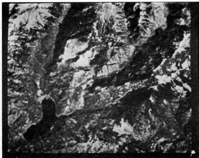
Figure 20a. Uncorrected Landsat Band 7 (0.8-1.1 \mu\text{m} ) imagery of the Vallecito Reservoir area in the San Juan Mountain test site.
