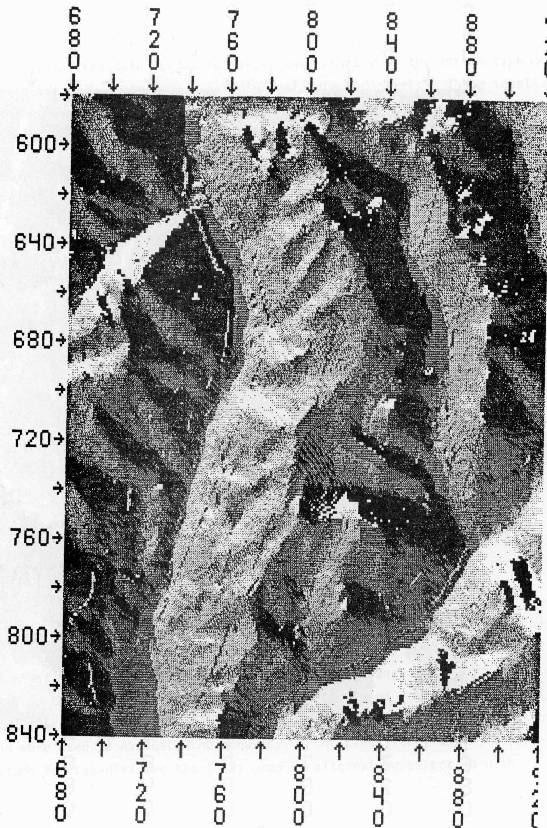
Figure 5a. Example of digitally interpolated aspect data for the same area shown in Figure 3. Aspects ranging from 0^{\circ} (North) to 360^{\circ} are displayed in shades of gray. Lighter tones are west and northwest-facing slopes.
