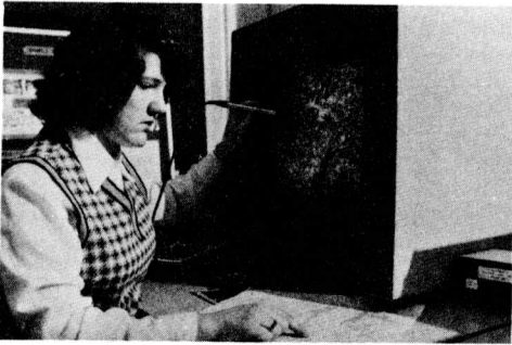
Figure 13. LARS Digital Display Unit with Light Pen for Interfacing with the Data.
