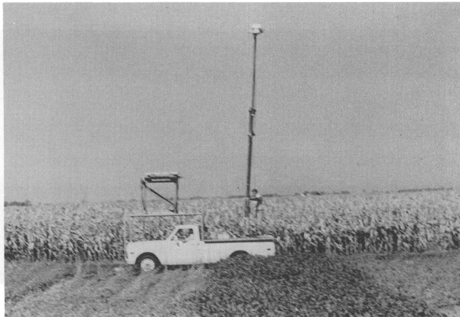
Figure 6. Truck-mounted boom positioning the multiband radiometer.
