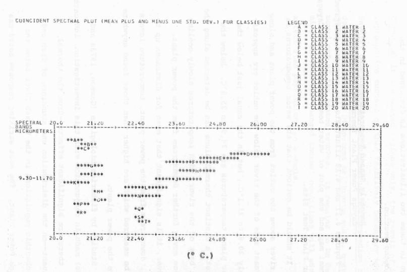
Figure 4.12. Plot of radiant temperatures corresponding to the areas outlined in Figure 4.11. The characters "A" through "T" indicate the mean temperatures and the length of the asterisks represent + 1 o.
