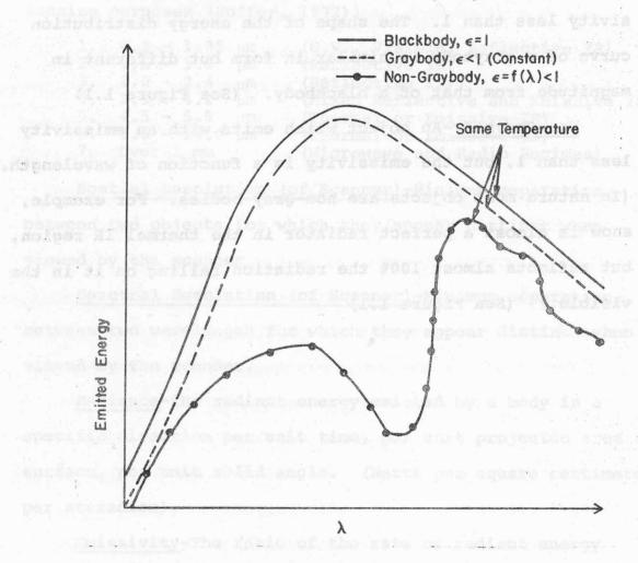
Figure 1.1. Comparison of the emissive characteristics of a blackbody, graybody and non-graybody over a range of wavelengths.
