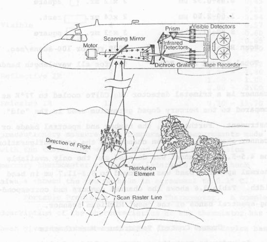
Figure 3.3. Schematic configuration of the "new" Michigan multispectral data collection system.
