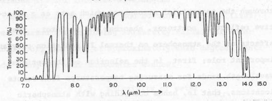
Figure 2.2. Transmission spectra of the atmosphere for 304 m. (1,000 ft.) path-length at sea level. Atmospheric windows in the thermal IR region of the spectrum.
