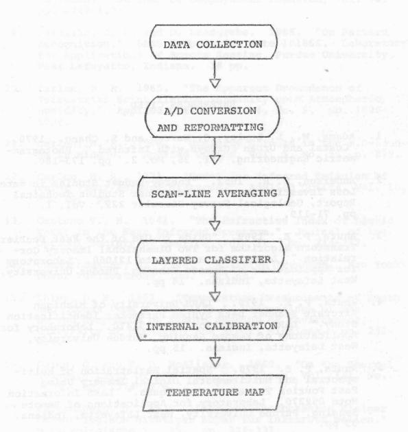
Figure 5.1. Recommended procedure-sequence for operational thermal mapping.
