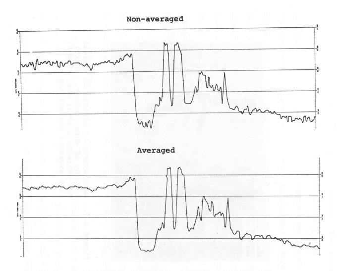
Figure 4.8. Graph of a scan line before and after scan-line averaging.
