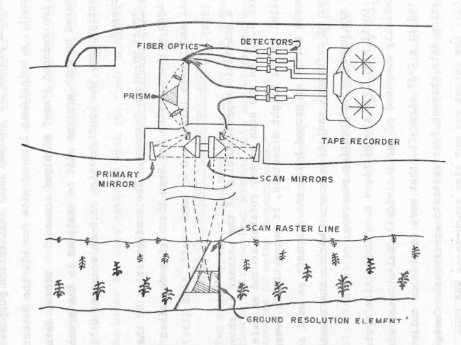
Figure 3.1. Schematic configuration of the "old" Michigan multispectral data collection system. [Illustration credit--R.A.Holmes]
