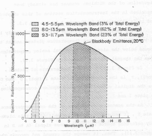
Figure 3.12. Percent radiant energy emitted by a blackbody in the 4.5-5.5, 8.0-13.5 and 9.3-11.7 micrometer spectral bands.
