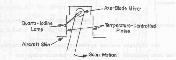
Figure 3.2. Schematic configuration of the Michigan thermal IR scanner.
