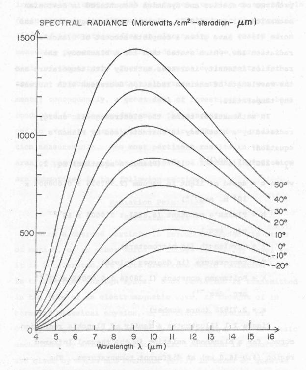
Figure 2.1 Planck's radiation curves for thermal emission from a blackbody at typical terrestrial temperatures.
