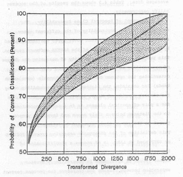
Figure 3.5. Empirical relation between transformed divergence and correct recognition (1-6 features). [Swain, 1973]
