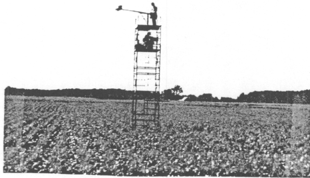
Figure A4.1. Reflectance factors were measured at many angles from the top of a 10 m tower.
