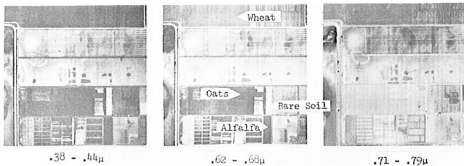
Figure 6. Multispectral response comparison of wheat, oats, alfalfa, and bare soil as of 1630 hours on 25 June 1964. The differences in relative response of bare soil in this figure as compared to Figure 5 are largely due to a difference in soil type.
