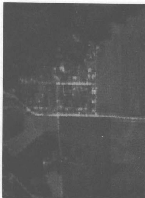
Figure 3.18. Reconstructed Channel 2 Image Using the K-L Encoder at Three Different Data Rates (8x8x1 Data Blocks).
