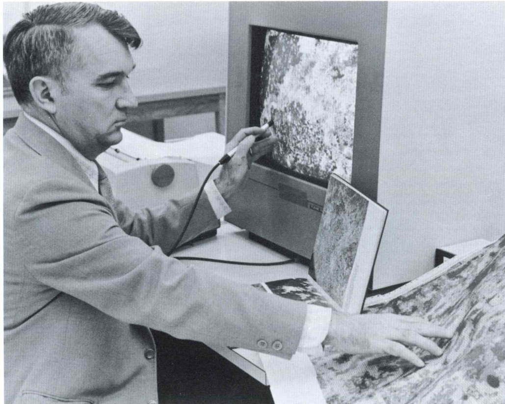
Figure 7 Special display systems such as this allow the operator to direct the computer's handling of image data. The light pen in the researcher's hand can be used to mark the screen, recording the address of a point or field of interest.
