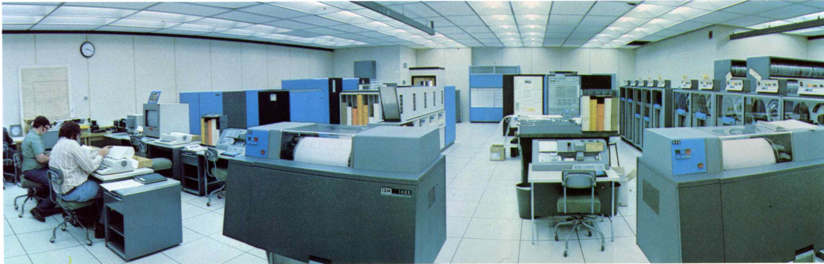
Figure 8 The LARS/Purdue computational facility, an IBM 360/Model 67 time-share computer with terminals for analysis of data on this system located in several other offices and laboratories across the country.
