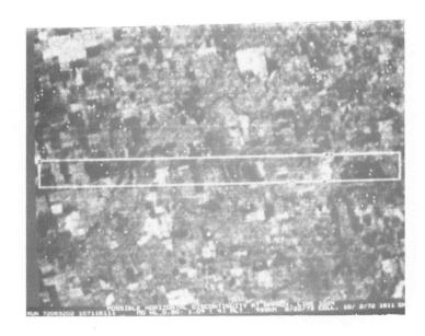
Figure 10.3 Horizontal discontinuity example in scene corrected data Frame 1071-16111-601. Band 7.
