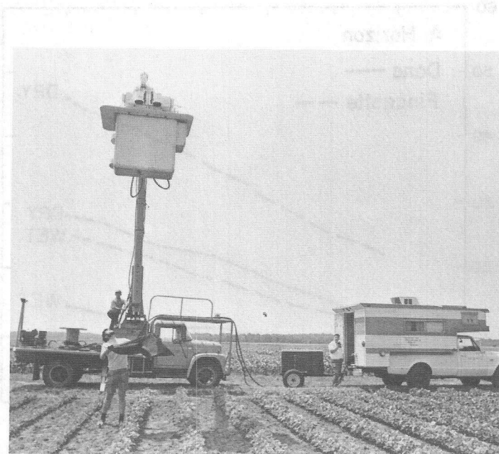
FIGURE 4. Long wavelength and short wavelength heads arranged in the foresighted mode for extended wavelength spectroradiometry.
