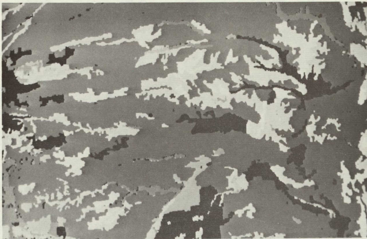
Figure 2.2b-9 Land use map classification processed by cleaning algorithm with parameter L = 2 .
