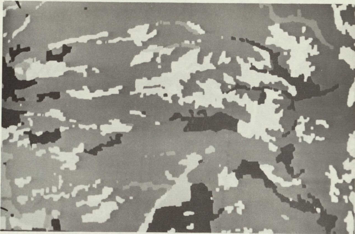
Figure 2.2b-11 Land use map classification processed by cleaning algorithm with parameter L = 4 .
