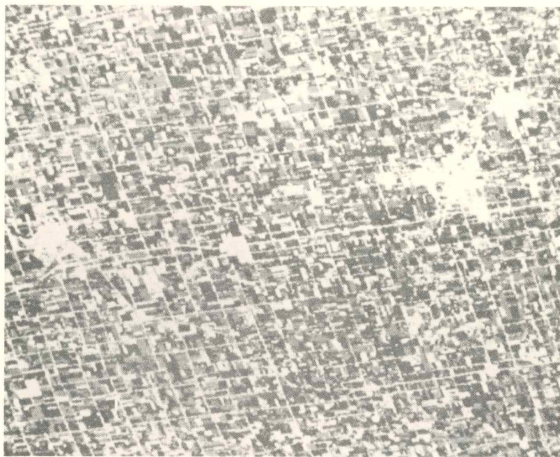
Figure 2. Computer classification map of corn, soybeans and "other." (Corn: black; soybeans: gray; "other" white.)
