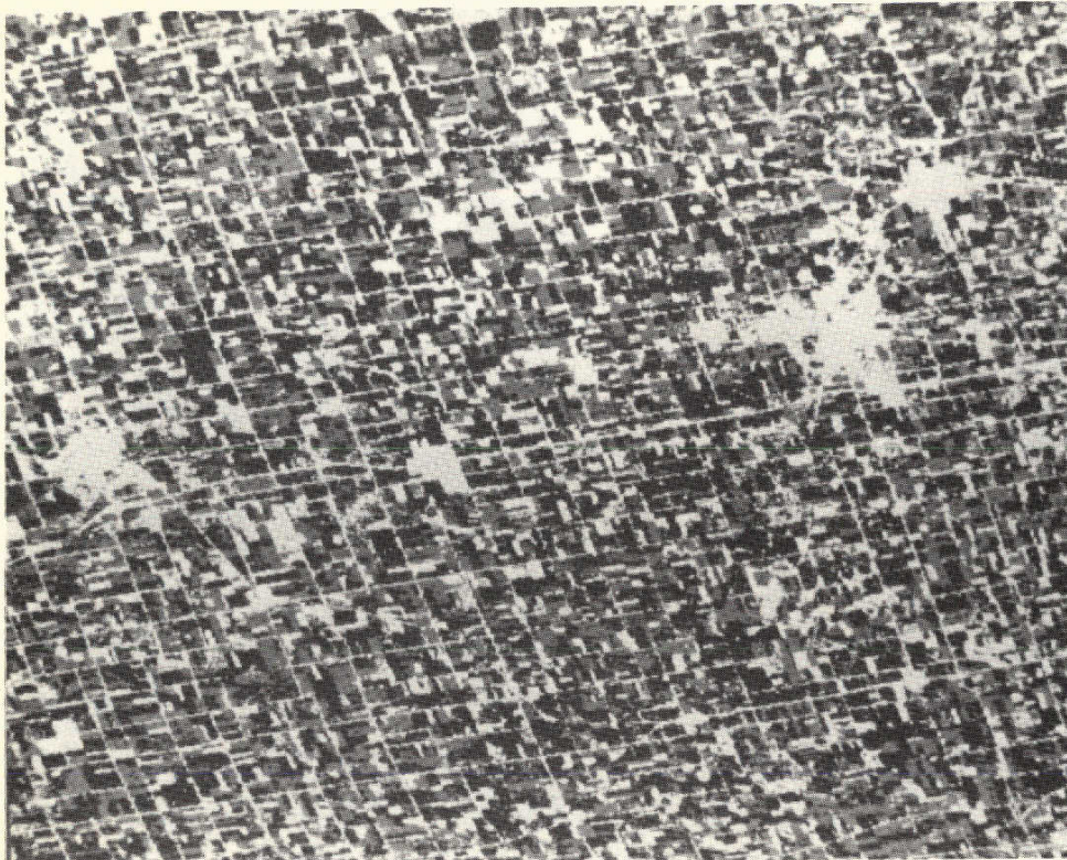
Figure 9. Computer Classification of ERTS Data Identifying Corn (Black), Soybeans (Gray), and all Others (White). (DeKalb Co., Illinois)
