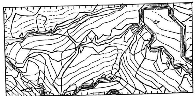
Figure D.4. Output of shadow mapping program showing areas having similar aspects.
