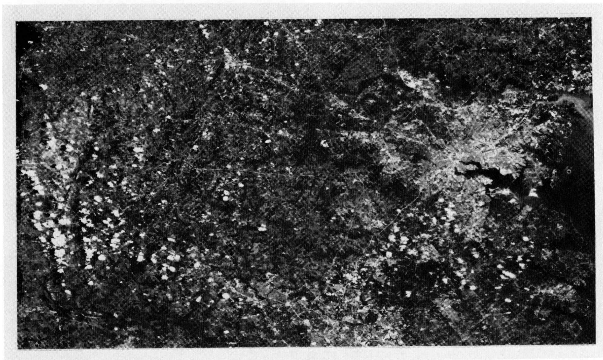
Figure 14. Frame mean/standard-deviation equalization on raw, uncalibrated data from Baltimore area of Scene 2904-14455, Band 4
