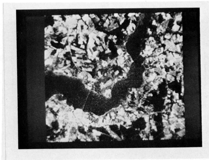
Figure B9. Gray scale image of Landsat spectral band 5, produced on the digital display.
