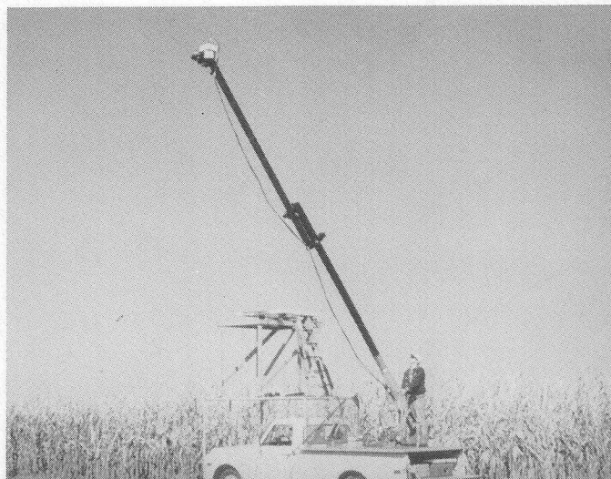
Figure 3. During the past several years an instrumentation system for acquiring reflectance and radiant temperature measurements of crop canopies and soils has been developed. The system includes a multiband radiometer, data logger, camera, calibration standard and aerial tower. In addition to the instrument configuration shown here, the radiometer and data logger can also be mounted in a helicopter or light aircraft to obtain multispectral data of commercial fields.
