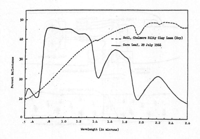
Figure 1 Reflectance Curve of dry Chalmers Silty Clay Loam and a Corn Leaf
