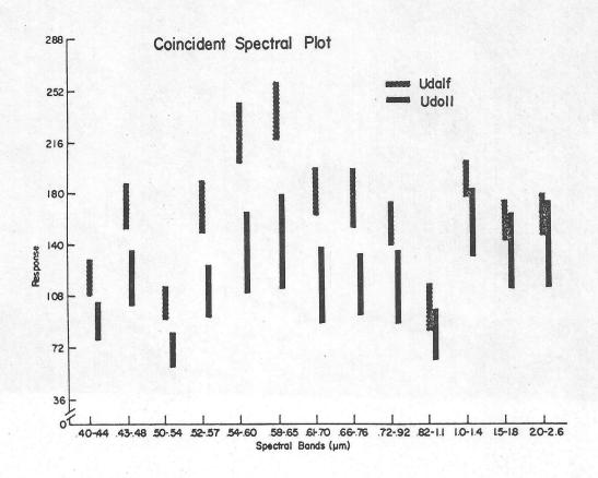
Figure 3 Coincident Spectral Plot Showing Higher Reflectance from Udalf than Udoll Soils over 13 Spectral Bands
