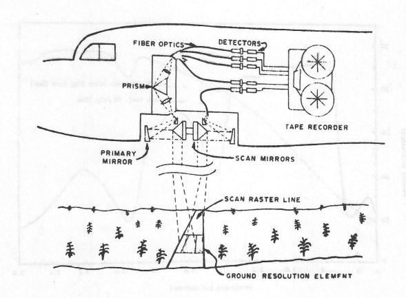
Figure 2 Single Aperture Multispectral Scanner
