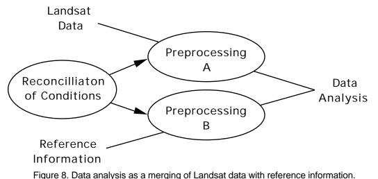
This Reference information can take a wide variety of forms. It can be in the form of quantitatively expressed reference spectra gathered for the classes present in the Landsat data, but at a previous time, and perhaps from laboratory or field measurements. At the other extreme, the required reference information can simply be input by the analyst, designating in the Landsat data set to be analyzed, example areas of each class of interest.
