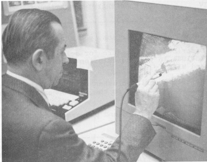
Figure 9 Analyst using a light pen to select training areas on a digital display
