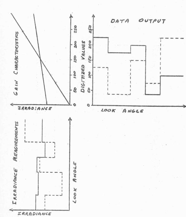
Figure 1. Gain Changes in Multispectral Data Handling System
