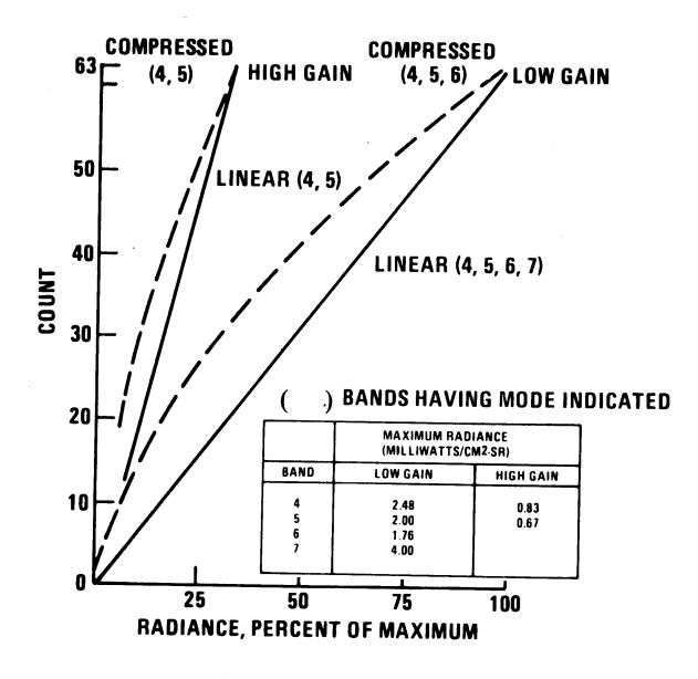
Figure 4. MSS Output vs Radiance, Compressed and Linear Modes.
