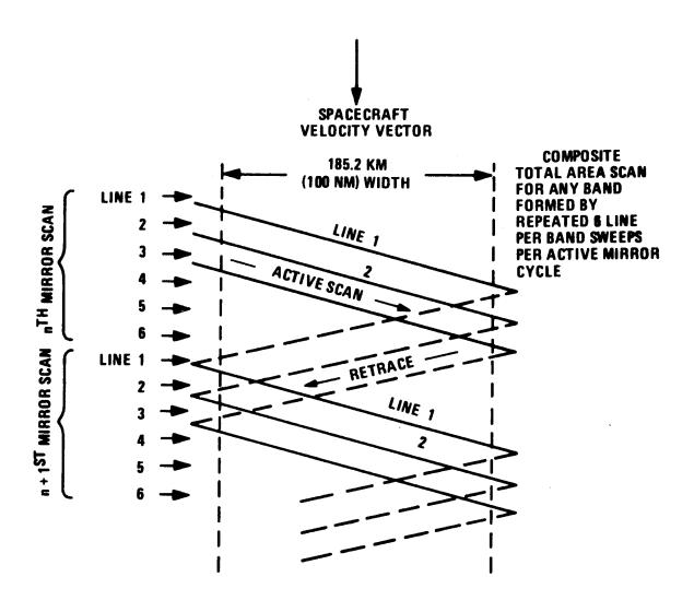
Figure 2. Ground Scann Pattern for a Single MSS Detector.
