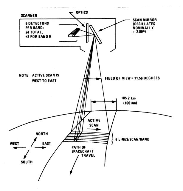
Figure 1. MSS Scanning Arrangement.
