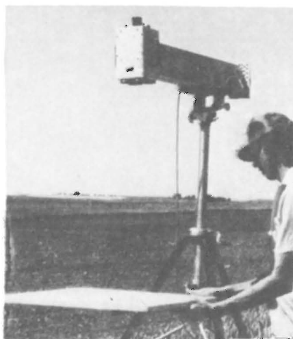
Figure 4. Tripod platform for Landsat band radiometer.
