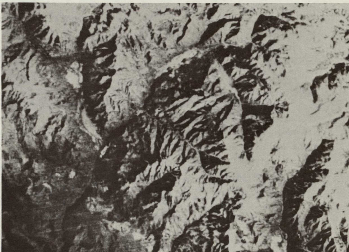
Figure E.6. East Fork landslide on the East Fork of the San Juan River. This landslide shows many of the diagnostic features such as a prominent scarp, undrained depressions, hummocky topography, deranged drainage, and disrupted topographic and vegetation patterns. The mottled appearance of the vegetation reflects the hummocky topography and unstable nature of the land mass. The diagnostic features are more easily detected when viewed in stereo. (LANDSAT scene 2222-17020, October 25, 1975)
