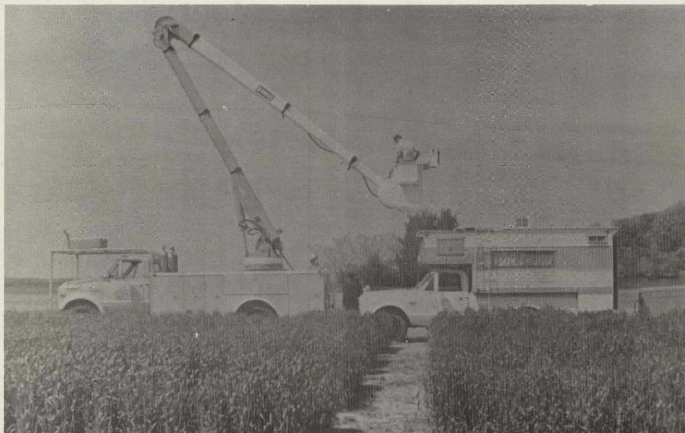
Figure 5.1.7 Typical Setup of the Field Spectroradiometer System
