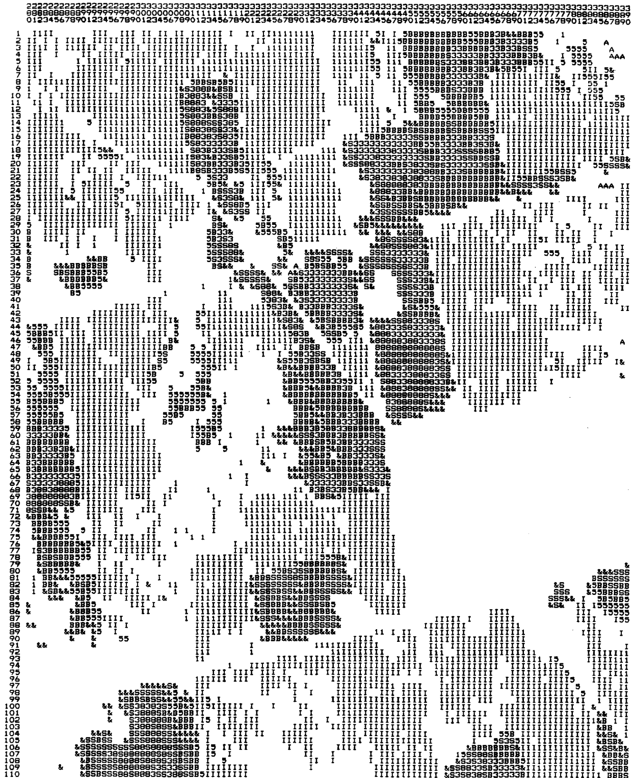
Figure V-5. A portion of the classification displaying two classes of corn (I,1), six classes of soybeans (S, 8, 3, B, 5, and &), and a wheat/residue class (A). All other classes are displayed by blanks.
