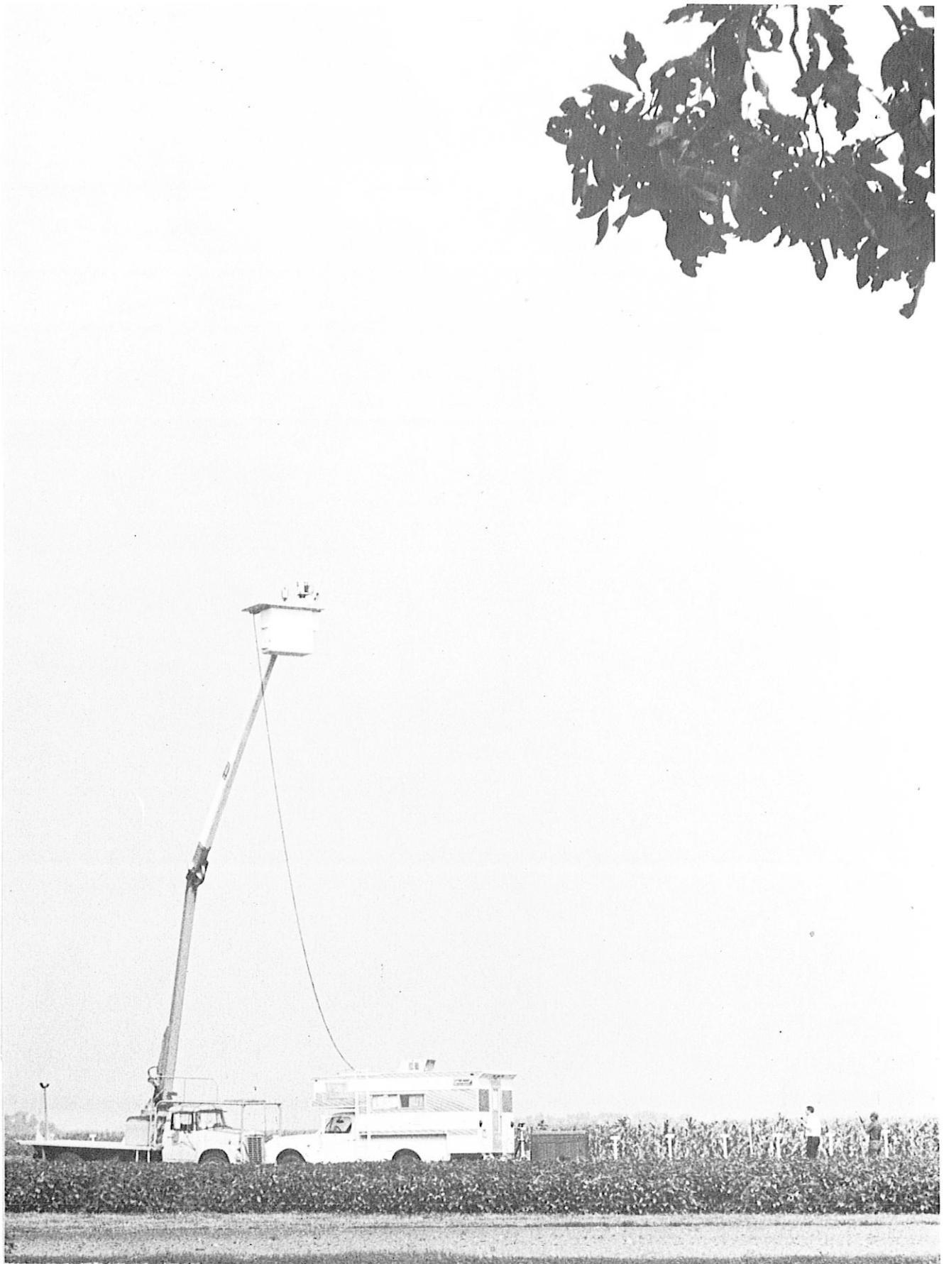
Figure 5 Measuring soybean radiance in both the 1 to 6\mu band (195E) and the 2 to 16\mu band (195T) from the cherry picker.
