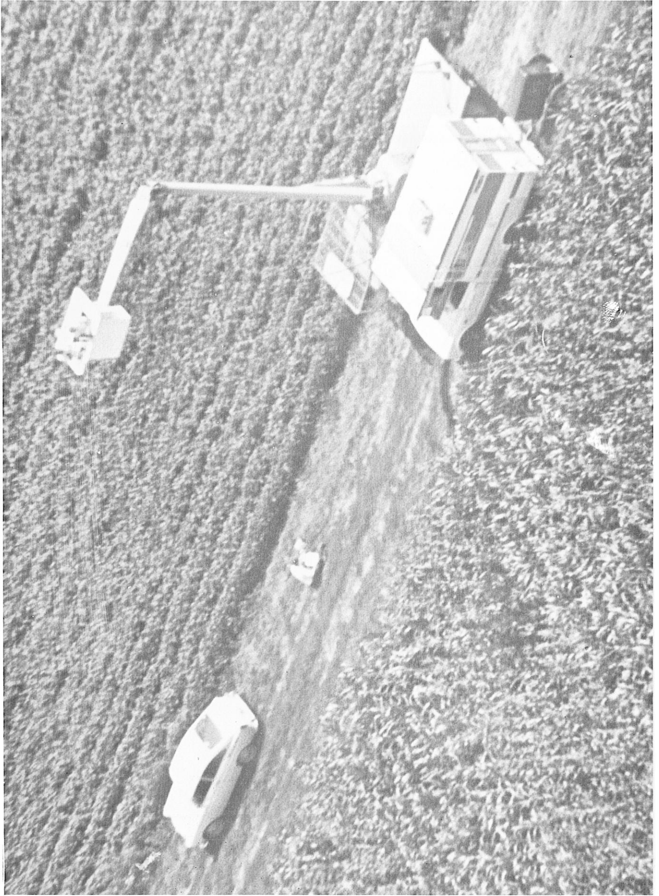
Figure 4 Measuring corn field radiance in the 2 to 16 \mu band from the cherry picker during a NASA flight mission.
