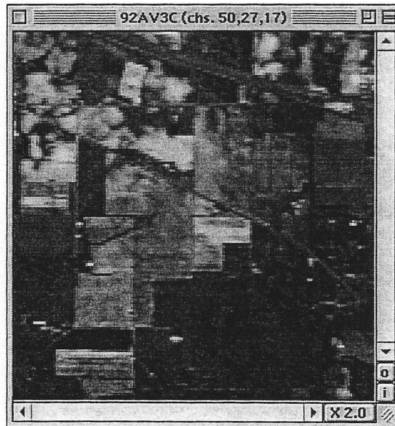
Figure 1. Example 3-channel color multispectral image from a 1992 AVIRIS data set. The 'i' and 'o' buttons are controls for zooming in and out respectively. The 'X 2.0' control indicates the current zoom factor and gives a quick way to go to a X1.0 zoom factor. One can zoom in 0.1 or 1.0 increments.
