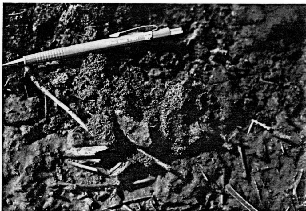
Figure 15. Loose, puffy and white-needle shape features of soils affected by Na_2SO_4 . (Photograph: Al-Mahawili, 1981)
