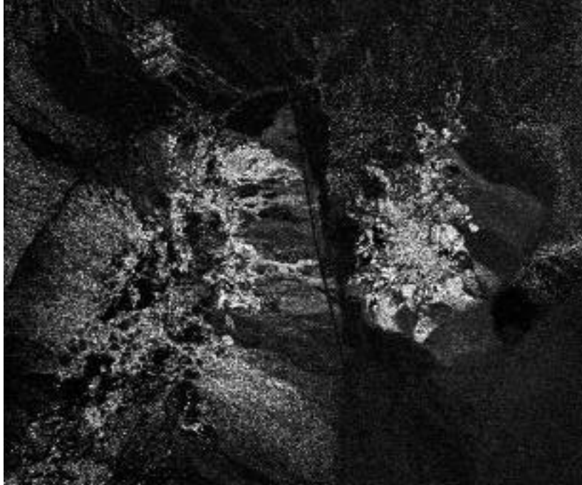
Figure 5. A Likelihood Map. Dark areas indicate low likelihood of membership in the class to which they have been assigned, while light areas indicate high likelihood.
