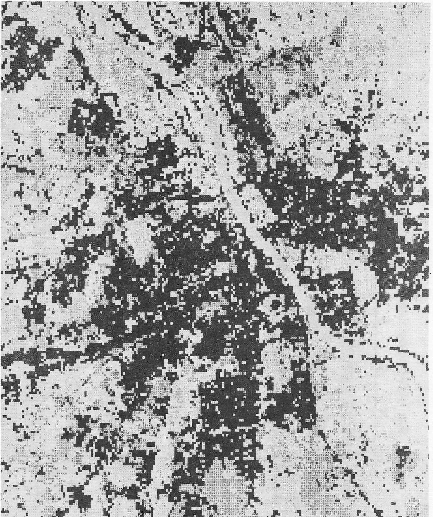
Figure 8. Printout classification map of Warsaw area using the electrostatic printer/plotter.
