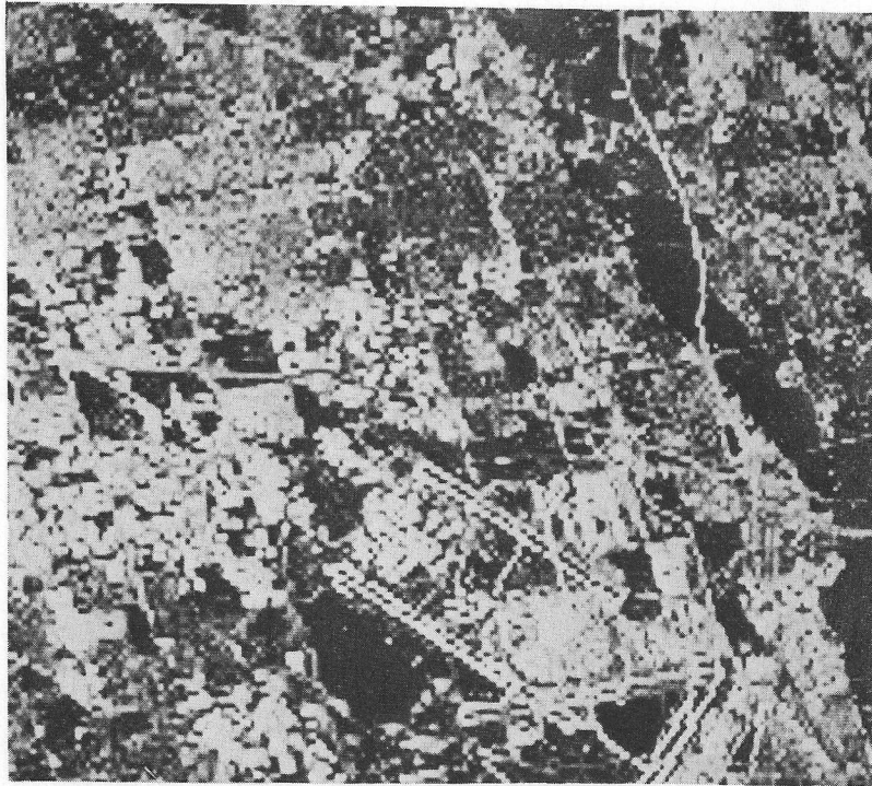
Fig. 10(e): An optimal IFOV enhancement of Fig. 10(a) using a restoration filter with a performance ratio of 0.45 and noise increase of 22 dB.
