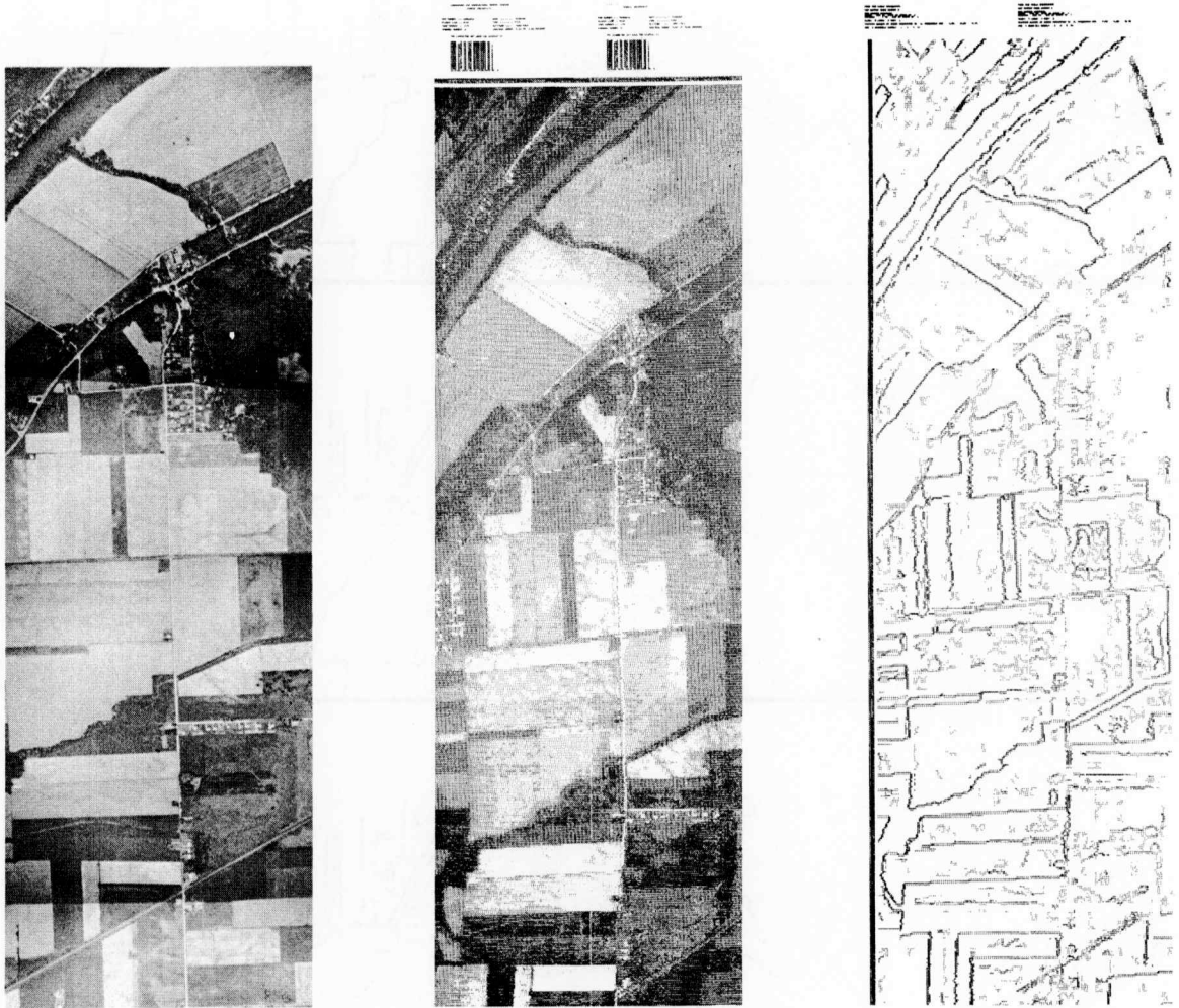
Figure 24-21.- Example output from the boundary-finding algorithm. An airphoto and line printer output are also given for comparison.
