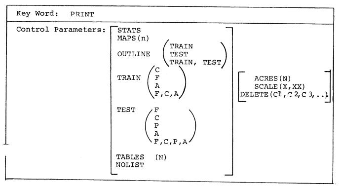
Function: Specifies printed output desired. Indicates which results tables are to be printed. Output includes channels used, classes, number of samples classified into each class, percentages of samples classified into each class, and an overall performance rating.
