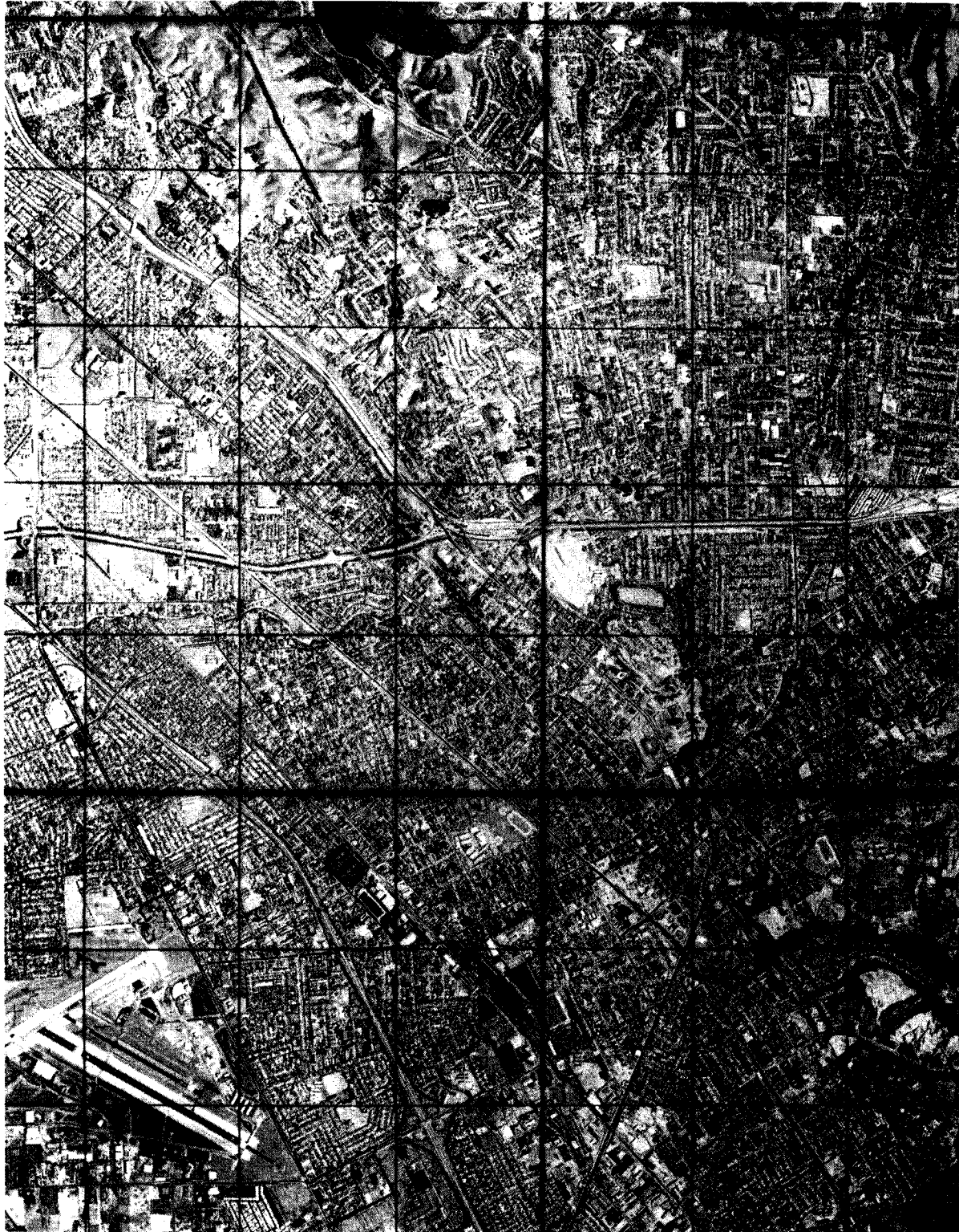
Figure 2. Black-and-white Photo of the Hayward Area, California. Photo by NASA for USGS Census Cities ERTS experiment: Zeiss camera, 12 in. focal length; 1:50,000 from RB-57 at 50,000 feet; color infrared film (S0-117), filter D; frame 252, 15 May 1970. Approximate orientation of one-kilometer UTM grid (zone 10) indicates scale, and facilitates comparison with corresponding computer land-use map.
