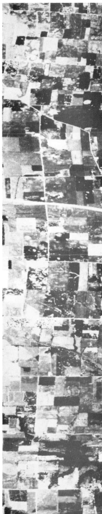
Figure 2. Aircraft Multi-spectral Scanner imagery (.58-.65 \mu band) showing severe geometric distortion due to crosswinds. LARS Run No. 71054100. Area is immediately west of Crawfordsville, Indiana. Date: August 17, 1971. Altitude: 5,000 ft.
