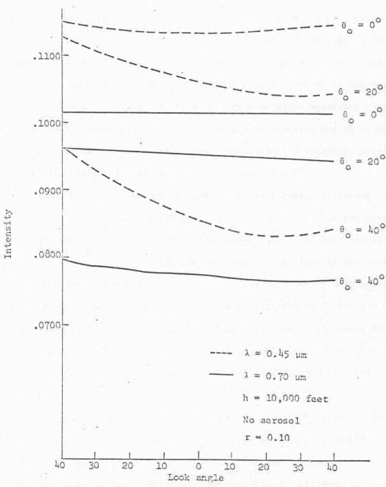
Figure 4-1 Intensity Modifications in a Rayleigh Atmosphere
