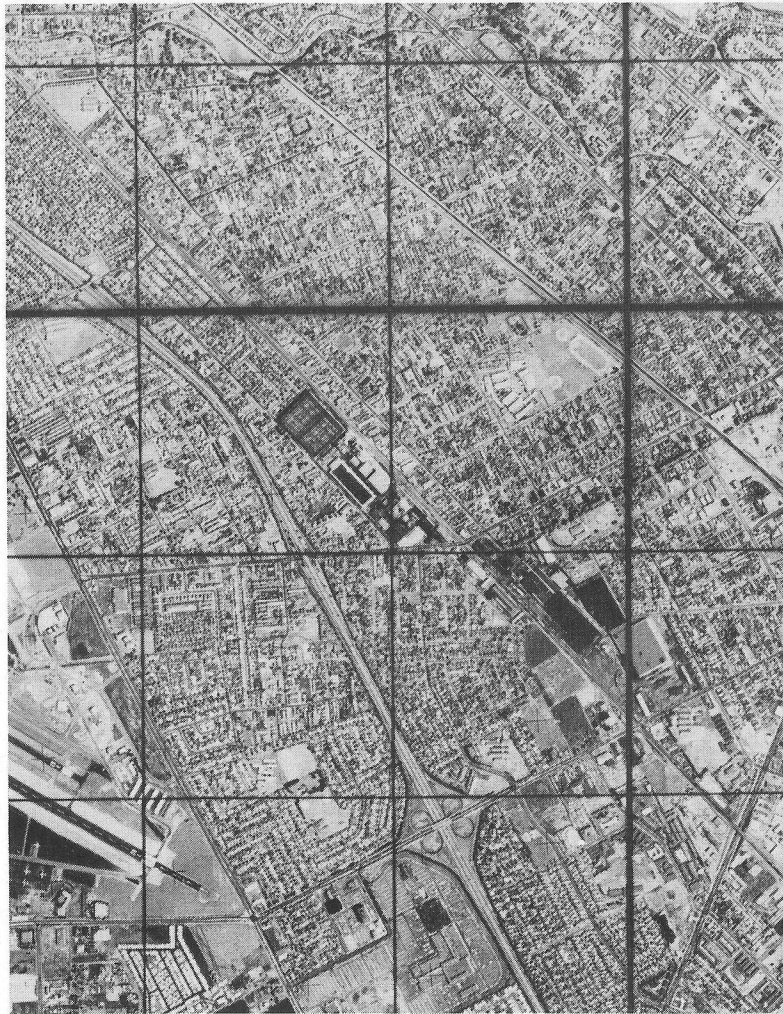
Figure 4 and Figure 5. Enlarged Photo-map Pair, Hayward Area, California. Photo is part of one high altitude color infrared scene acquired at 1:50,000, 15 May 1970, by NASA for USGS Census Cities ERTS experiment. Map is by Purdue/LARS and is based on ERTS-1 scanner digital data for frame 1003-18175, 26 July 1972. Scan lines have been reformatted so that they are nearly parallel to east-west UTM one-kilometer grid lines (zone 10). One printout symbol represents one ERTS scanner picture element (pixel), 0.465 hectare, or 1.1 acres. Urban classes: Commercial-Industrial (I); Mobile Homes (V); Residential (M); Parking Lots (.). Note correspondence between photo and map in mobile home area, lower left corner. Expansion of mobile home park (symbol V on ERTS computer map) is confirmed by NASA 1972 air photo.
