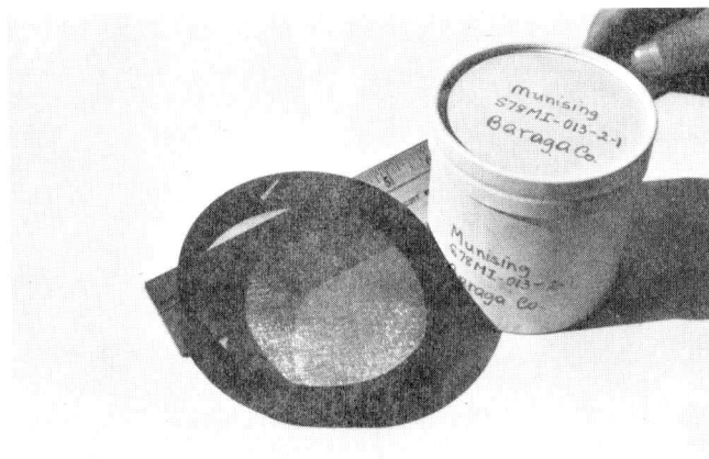
a. Soil sample and 10 cm diameter sample holder.
