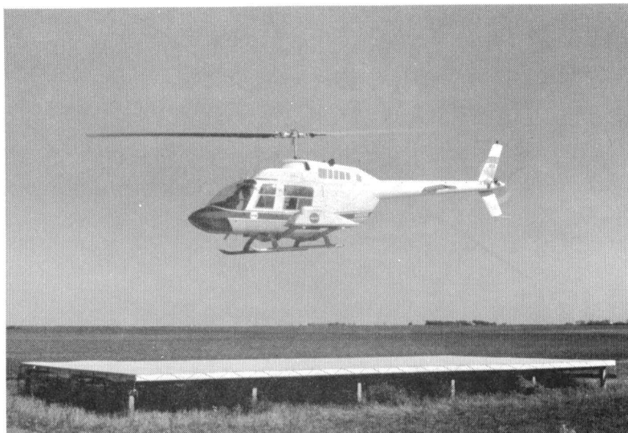
Figure 21. Helicopter equipped with spectroradiometer hovers at calibration site panel.
