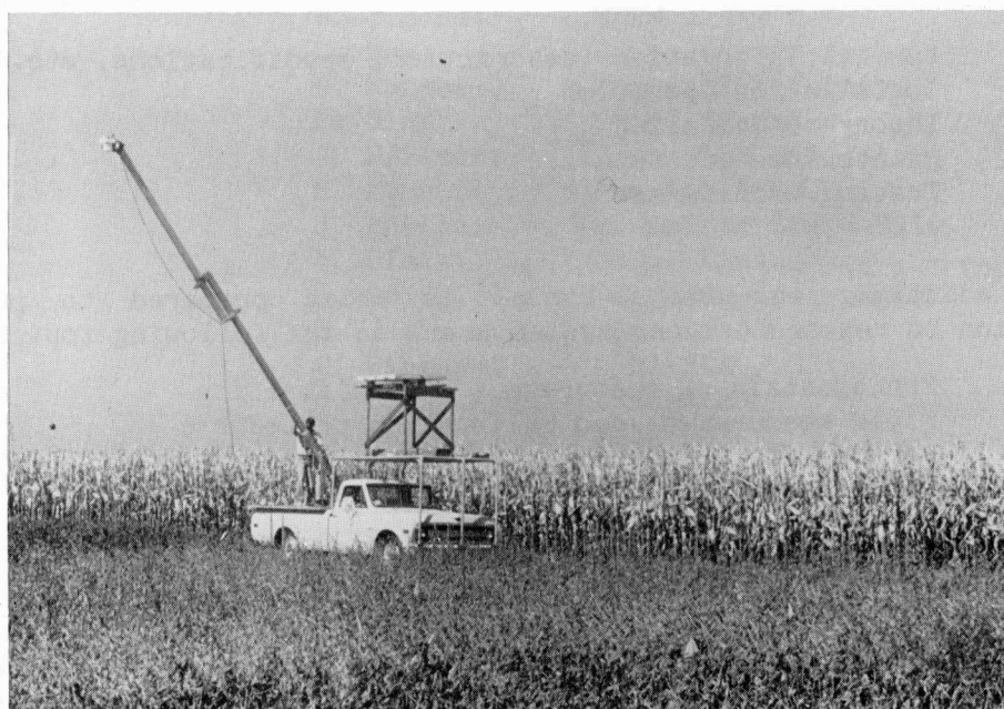
Figure C-16. Truck-mounted boom positioning the multiband radiometer.
