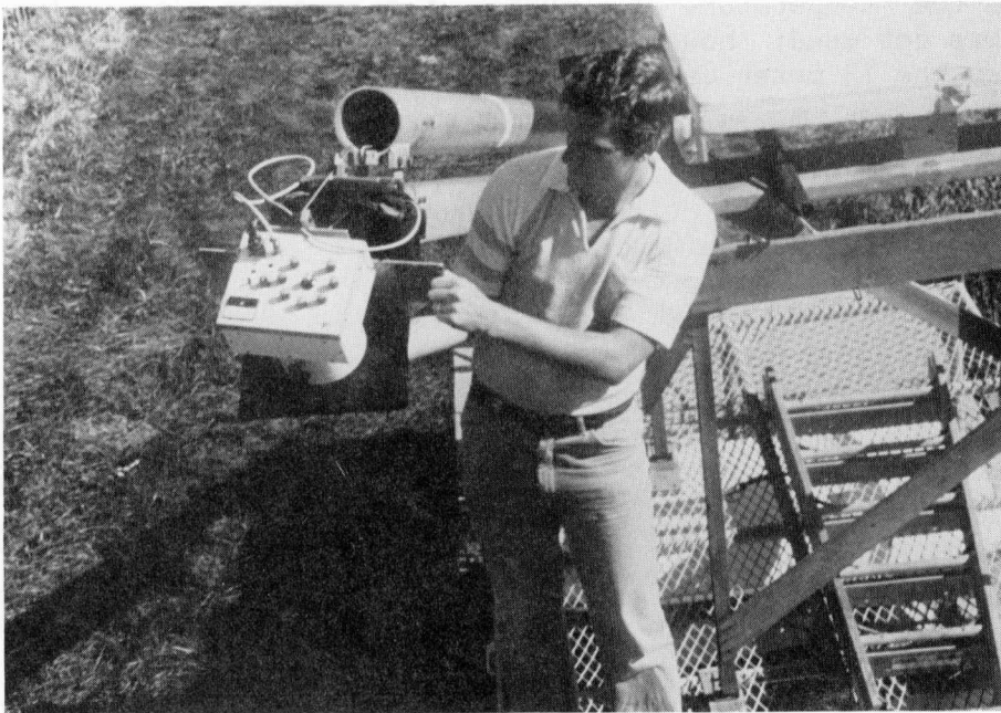
Figure C-13. Measurement of dark level response of multiband radiometer.
