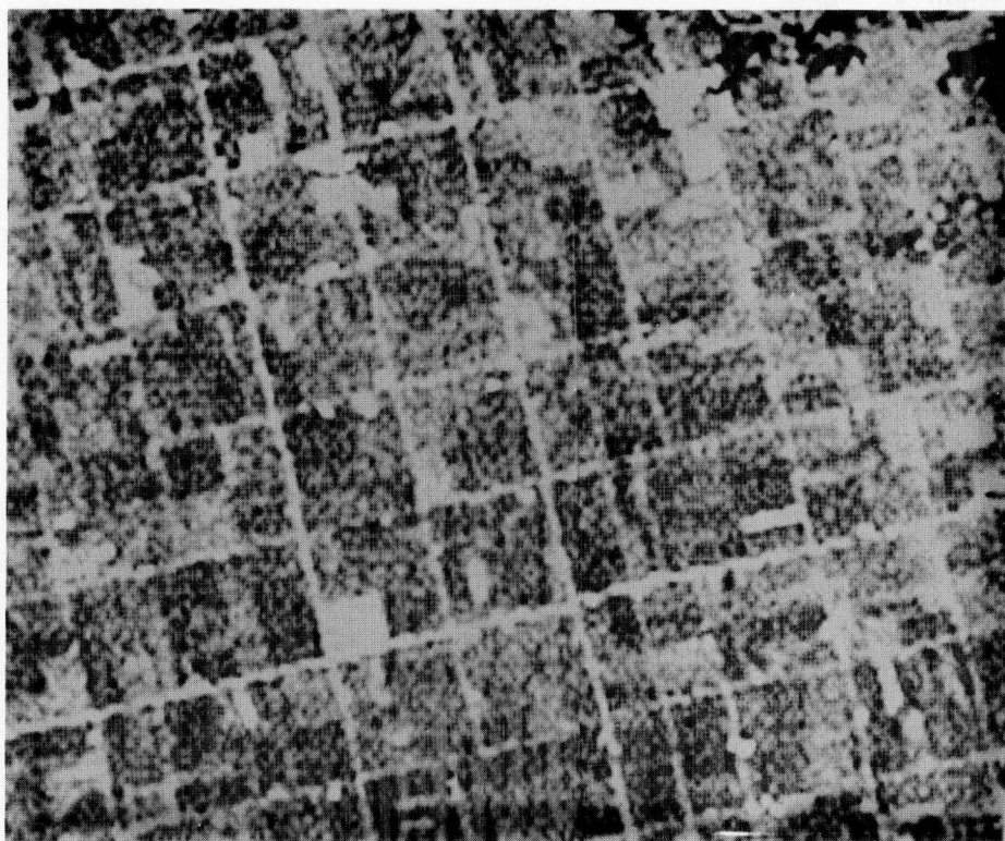
Figure 13-4. MSS band 5 imagery interpolated to 19m using cubic interpolation, September 3, 1980.
