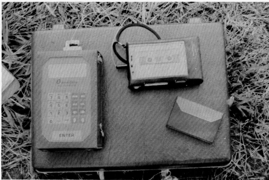
Figure 4-4. Model 516 Polycorder downloading to cassette tape--in the field.
