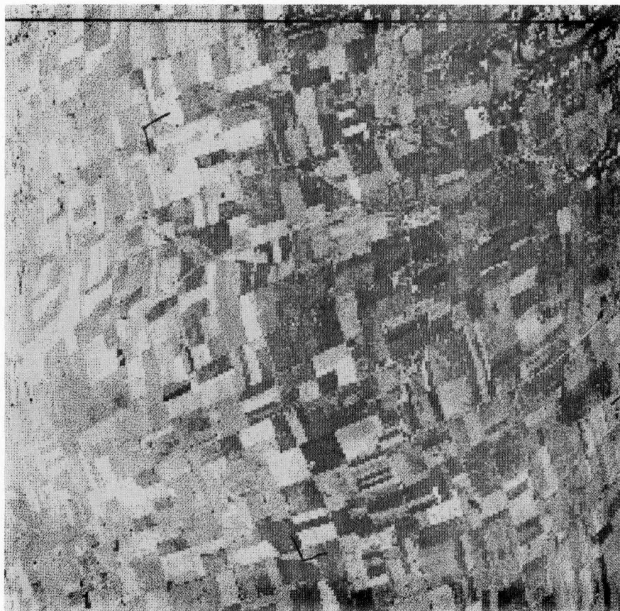
Figure 16-3. Webster County scanner data (1.0-1.3 \mu\text{m} wavelength band) for September 10, 1980 as received; every sixth scan line and third sample (column) shown.
