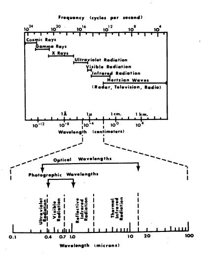
Figure 1. The electromagnetic spectrum. Note the relatively small range of wavelengths to which our eyes are sensitive.
