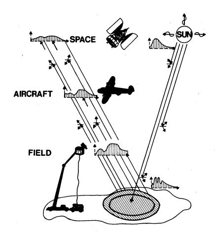
Figure 2. Multiple Levels of Research in Remote Sensing. Detailed field and laboratory studies on the spectral characteristics of materials of interest is extremely important in order to more accurately interpret the remote sensor imagery from aircraft and spacecraft.
